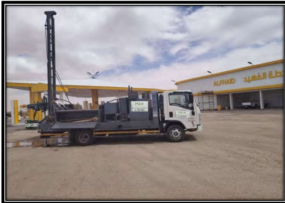
Truck Mounted Drilling Rig -02
